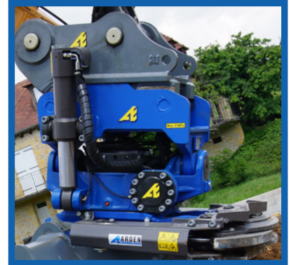
AIO with ATR: full rotation and tilt on both sides.
